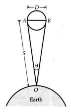
**Radar method:** The word RADAR stands for *radio detection and ranging*. A radar can be used to measured accurately the distance of a nearby planet (such as Venus). Here radio waves are sent from a transmitter which after reflection from the planet are detected by the receiver. By measuring the time interval (t) between the instants the radio waves are sent and received, the distance of the planet can be determined as
