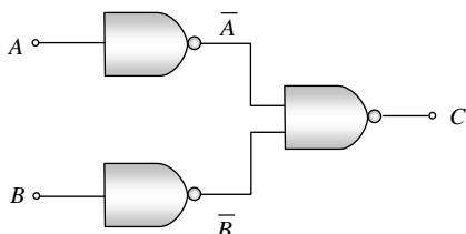
$$C = \overline{A \cdot B} = \overline{\overline{A} + \overline{B}} = A + B \text{ (De morgan's theorem)}$$
