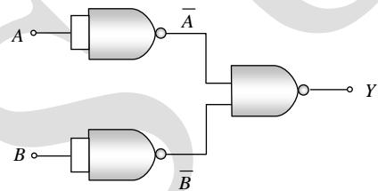
$$Y = \overline{A \cdot B} = \overline{\overline{A} + \overline{B}} = A + B$$
