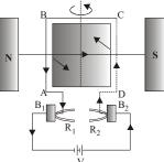
Split-rings or Commutator : These are two halves of the same ring. The ends
