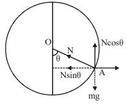
As  $|\cos \theta| \le 1$  therefore the bead will remain stuck to its lowermost position, provided  $\frac{g}{R}\omega^2 \le 1$
