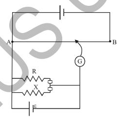
Figure shows a 2.0V potentiometer used for the determination of internal resistance of a 1.5V cell. The balance point of the cell in open circuit is 76.3 cm. When a resistor of  $9.5\Omega$  is used in the external circuit of the cell, the balance point shifts to 64.8 cm length of the potentiometer wire. Determine the internal resistance of the cell.
