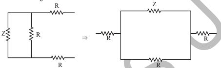
Adding of these resistors will not change the value of Z because the network is infinite then
