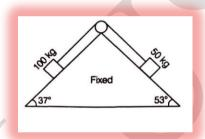
20. All strings are massless and pulleys are fixed and smooth. Find acceleration of blocks.
