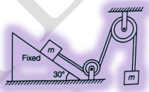
21. All strings are massless and pulleys are fixed and smooth. Find acceleration of blocks.
