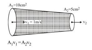
$$v_2 = \frac{A_1 v_1}{A_2} = \frac{10 \text{ cm}^2 \times 1 \text{ m/s}}{5 \text{ cm}^2} = 2 \text{ m/s}$$
